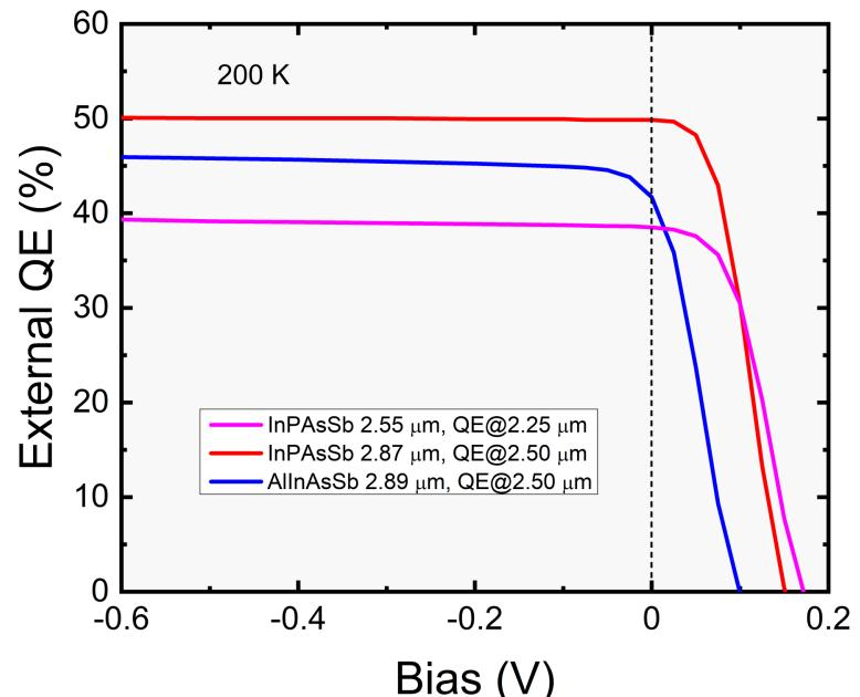
Sharp cutoff for longest-wavelength devices, softens for shorter wavelengths
