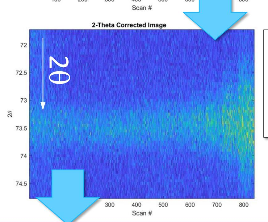
Scans are smoothed to enable improved fitting and determination of  $2\theta$  shift with scan number ( $\chi$ ).
