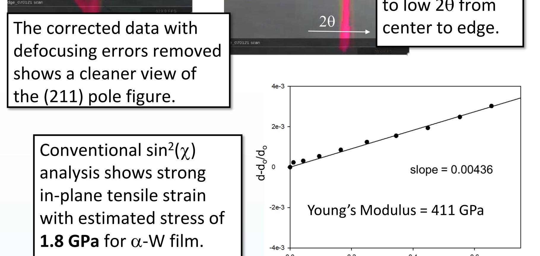
Conventional  $\sin^2(\chi)$  analysis shows strong in-plane tensile strain with estimated stress of 1.8 GPa for  $\alpha$ -W film.
