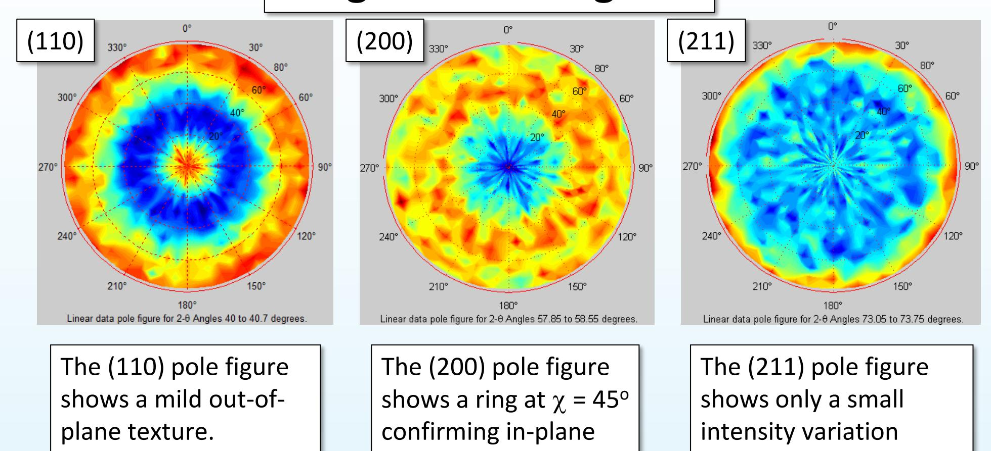
The (110) pole figure shows a mild out-of-plane texture.
