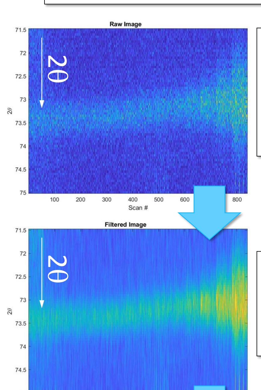
This plot shows all 840 XRD patterns measured for the (211) peak. This series shows a clear shift to lower  $2\theta$  values with increased  $\chi$  (i.e. scan #).
