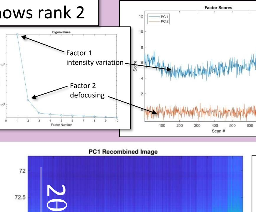
Principal Component Analysis shows Factor 1 as isolated peak for  $\alpha$ -W (211) and Factor 2 as defocusing.
