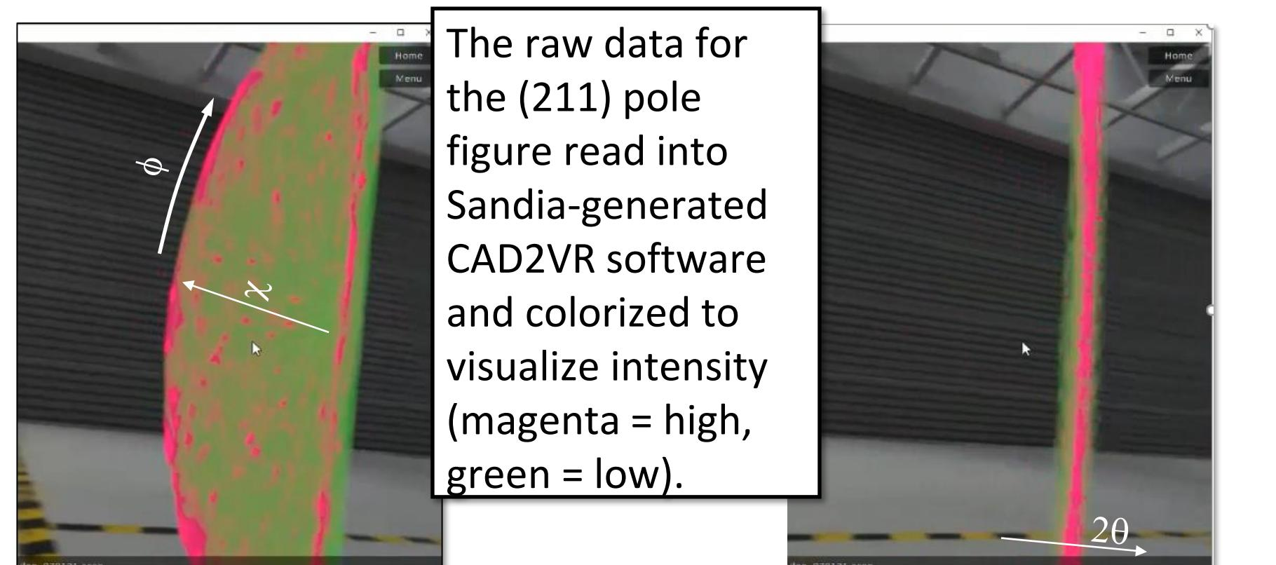
The raw data for the (211) pole figure read into Sandia-generated CAD2VR software and colorized to visualize intensity (magenta = high, green = low).
