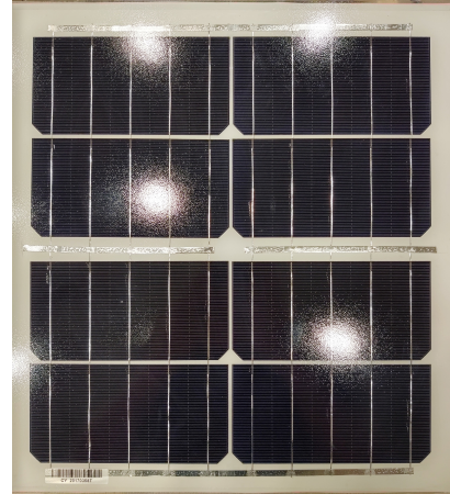
Fig. 1: Image of the front side of a half-cell minimodule. The module is divided into four pairs of cells that can be measured individually or as a whole module. Junction boxes connect to the tabs between each cell pair.
