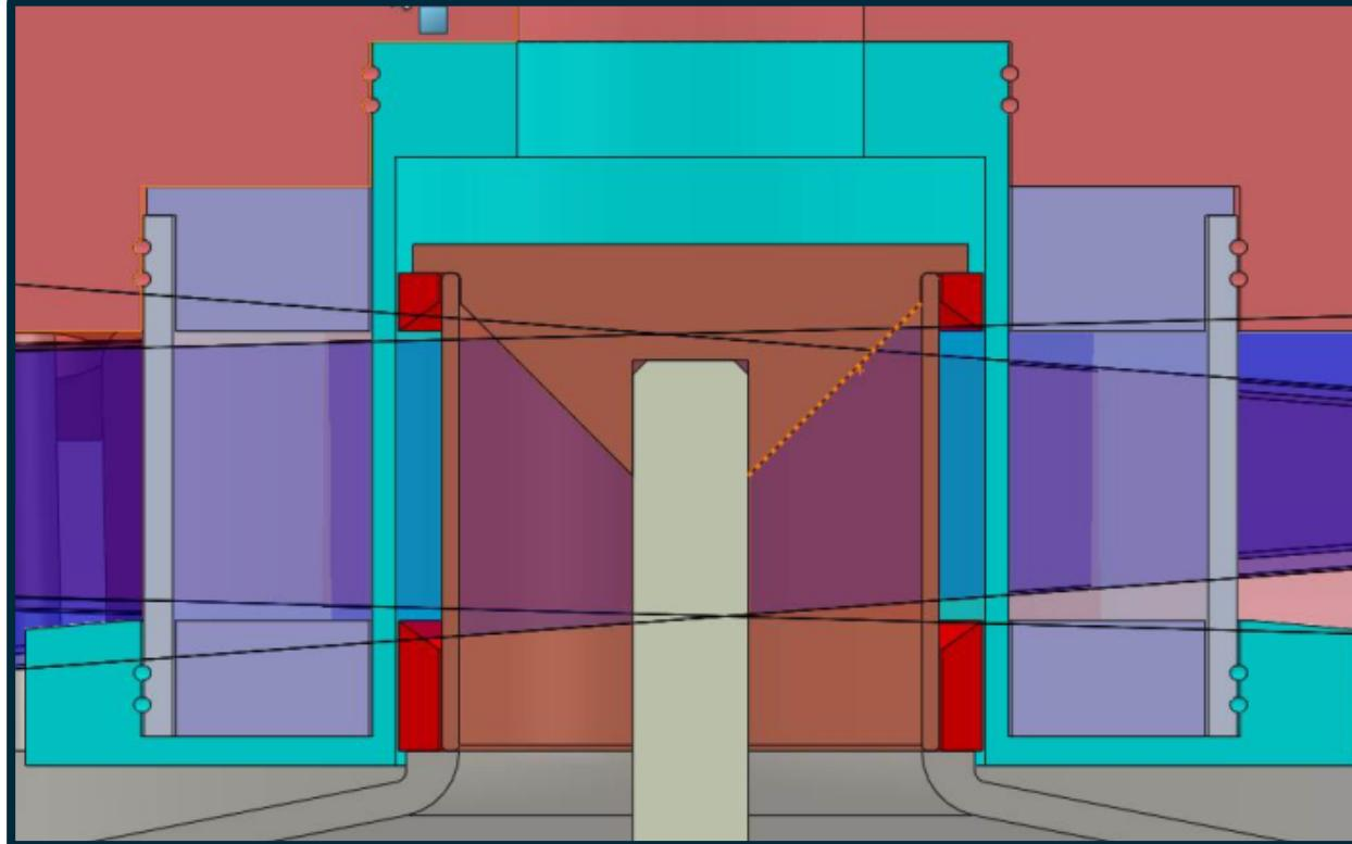
Glide planes were designed to minimize the impact of the wall instability
