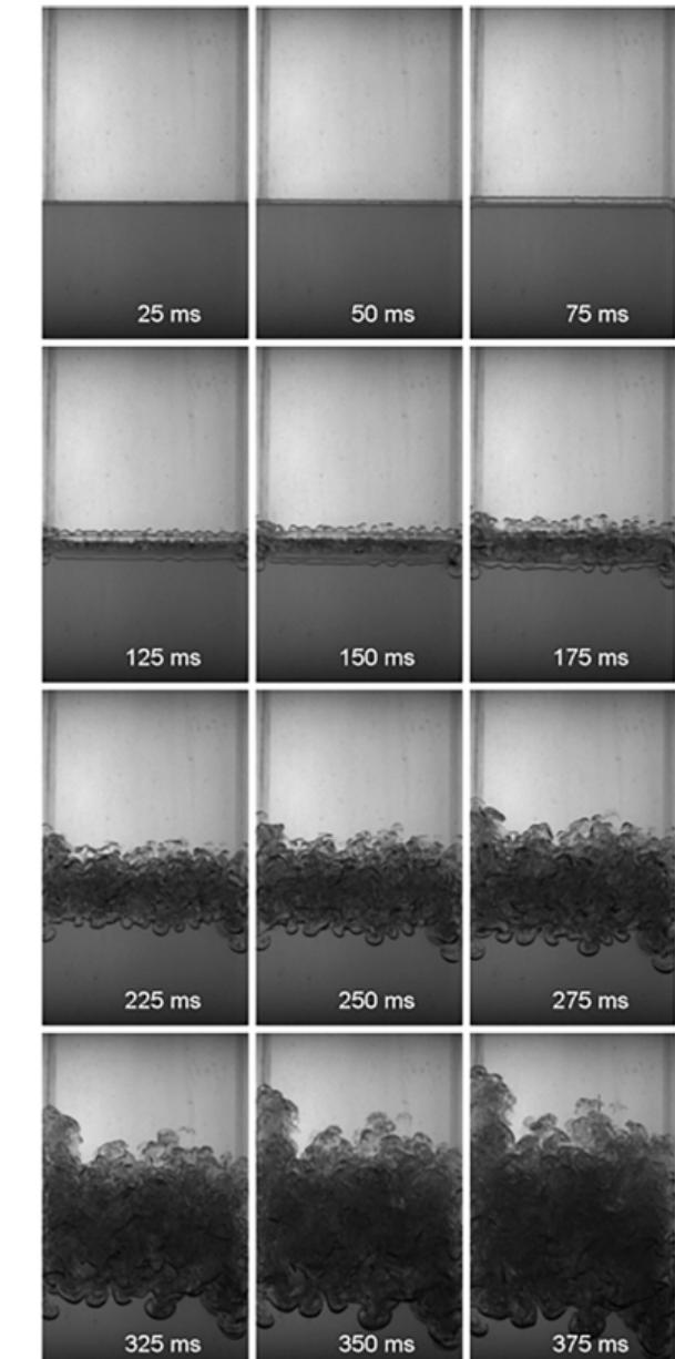
The exploding cylinder is an analog of the planar shock tube experiments which exploits cylindrical symmetry to eliminate limiting edge waves
