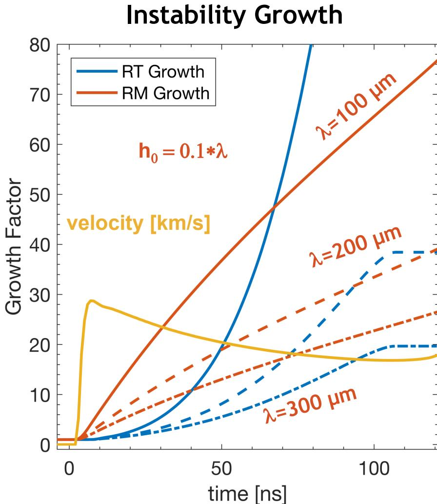
$$G_{\text{RT}}(t) = \exp \left( \int_0^t \gamma_{\text{RT}}(t') dt' \right) \quad \gamma_{\text{RT}} \approx \sqrt{-k_z A_N \frac{dv_i}{dt'}}$$
