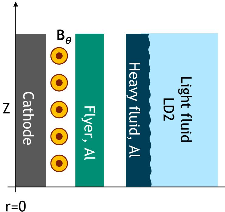
Cylindrical symmetry eliminates transverse edge waves and allows for Abel inversion to get quantitative densities. Given Z's long drive duration and energy, the practical limits to the experiment are the height and the radial size of the target
