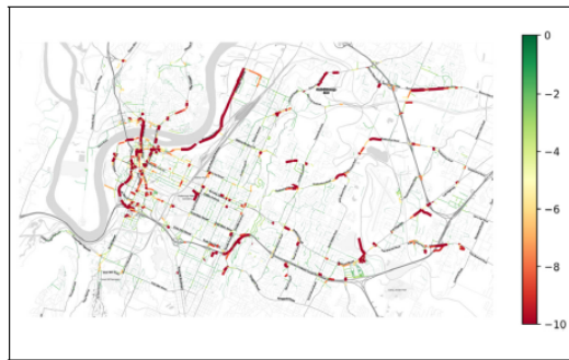
Figure 11. Link-level energy loss (gasoline gallon equivalent [gge] per mile) attributable to evening peak hour congestion.
