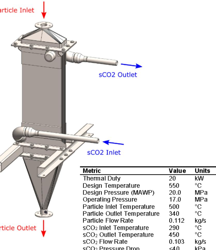
Prototype heat exchanger was developed to evaluate novel design features in G3P3:
