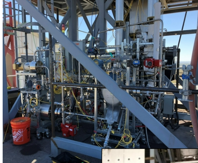
~100 kW sCO 2 flow loop
