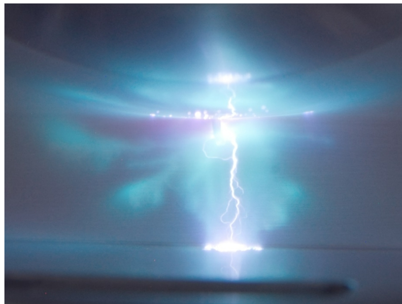
Selected breakdown triggered off thin wire representing a large defect
