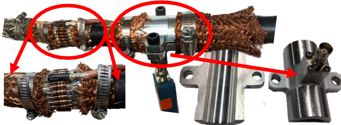
Current Viewing Resistor ~ 50 mΩ
