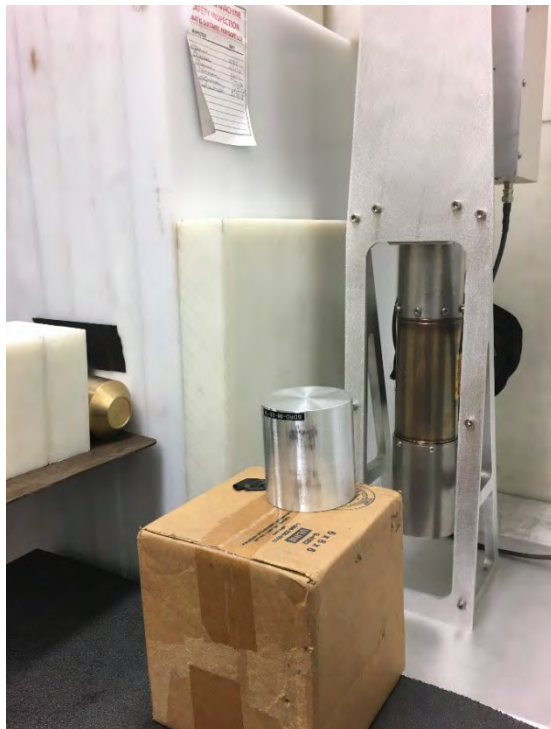
Figure 9. Experimental setup with Aluminum target facing STL API-120 STNG Tube, and CLYC detector.
