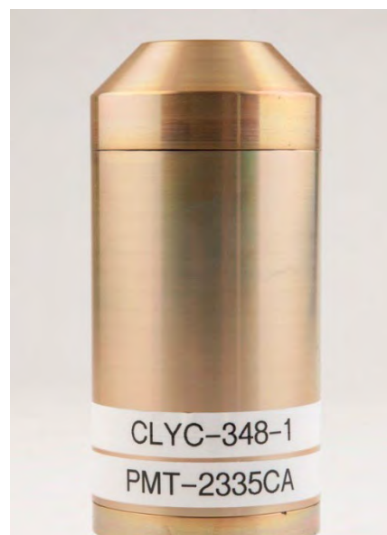
Figure 3. Elpasolite detectors were used to detect both neutrons and gammas.
