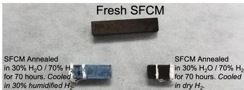
Figure 53. Photograph showing a fresh pressed and sintered bar of SFCM, and similar bars annealed in 30% steam (balance H_2 ) for 70 hours, where one was cooled in dry H_2 (right, no white precipitates) and the other was cooled in 30% humidified hydrogen (left, white precipitates).
