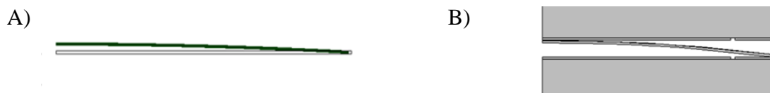
Figure 85. Curvature of a A) half-cell at room temperature after sintering and B) the cell placed in a stack assembly with curvature magnified 10x.
