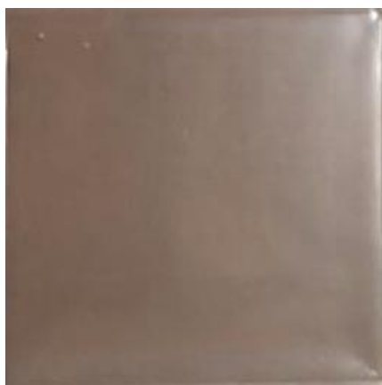
Figure 107. Example of 5 cm by 5 cm SFCM-based ceramic anode half cell without cracks as a result of an optimized firing profile and improved temperature uniformity in the furnace.
