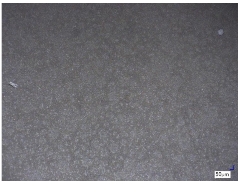
Figure 47. An optical image of the AFL surface of 5 cm by 5 cm SFCM-based ceramic anode cell #9 (sintered at the higher temperature) after test in which the electrolyte and cathode have peeled off completely.
