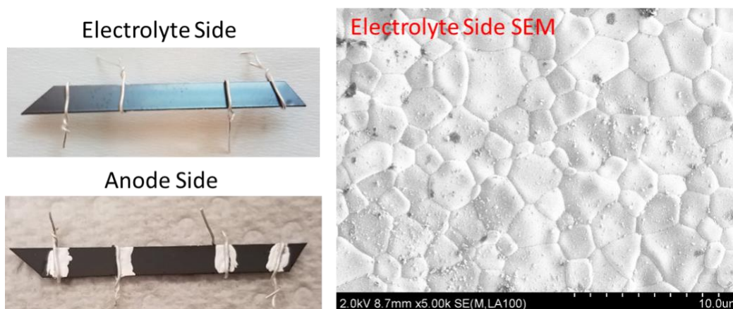
Figure 14. Sample 1 from Table 2 after measurement, showing no evidence for cracking after red-ox cycling.
