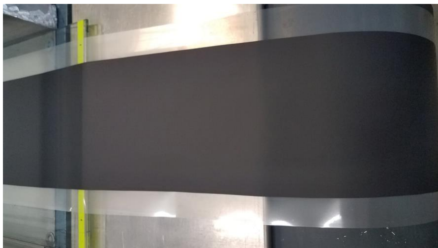
Figure 108. Photograph of a thinner SFCM-based ceramic ASL tape that enabled the fabrication of larger batch sizes as the tape dried more quickly and was able to be rolled up at the end of the pilot-scale tape caster, as shown on the right side of the image.
