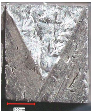
Figure 27. Fracture surface of single-phase dense SFCM bar, showing the notched areas (bottom left and right triangle features) and the region fractured during the test (i.e., top triangle area).
