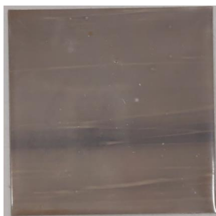
Figure 109. Sintered 5 cm by 5 cm SFCM-based ceramic anode half cell made with thinner ASL was found to be flat and without cracks.
