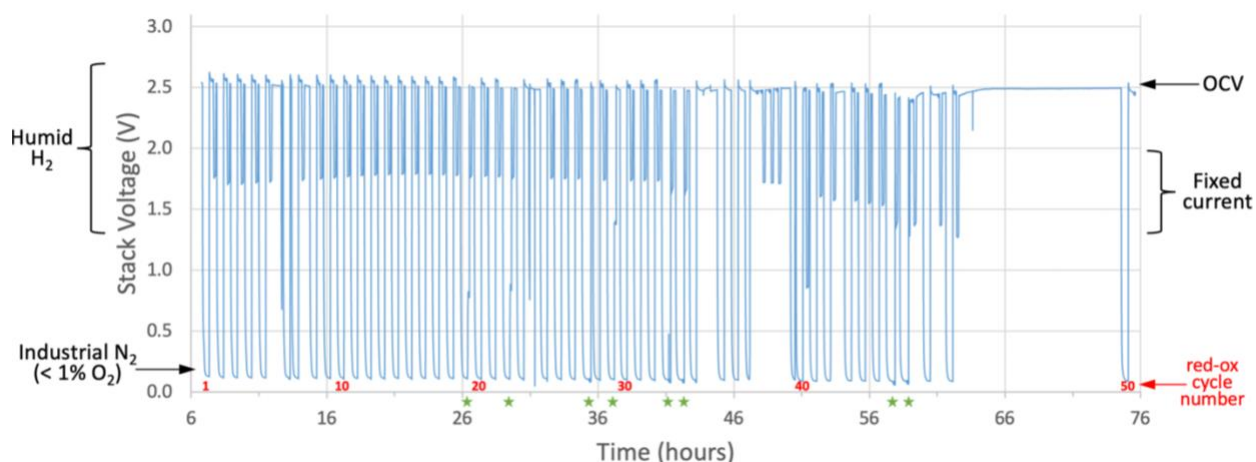
Figure 101. Stack voltage versus time for 3-cell stack using 5 cm by 5 cm SFCM-based ASL with AFL ( higher GDC content AFL at the higher sintering temperature ) and operating at \sim 600^\circ\text{C} during 50 red-ox cycles, switching between humidified \text{H}_2 and humidified industrial \text{N}_2 ( < 1\% \text{ O}_2 ) — the fixed current in \text{H}_2 was 0.21 \text{ A/cm}^2 , but green stars indicate when current was accidentally loaded to as high as 0.6 \text{ A/cm}^2 .
