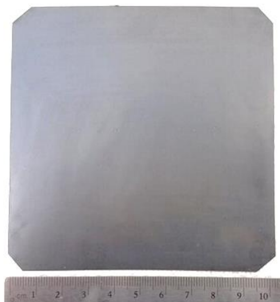
Figure 105. Example of 10 cm by 10 cm SFCM-based ceramic anode supported half cell with the anode and electrolyte co-fired at high temperature.
