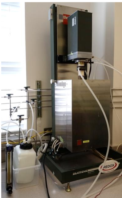
Figure 12. Redox's vertical pushrod dilatometer with atmosphere control for oxidizing and reducing conditions and more generally acquiring sintering curves and coefficients of thermal expansion for cell materials and stack components.
