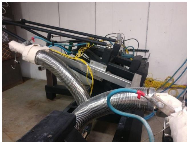
Figure 6: RF-Triple™ without Receiver tube thermal expansion component, extended to nearly 180° rotation
