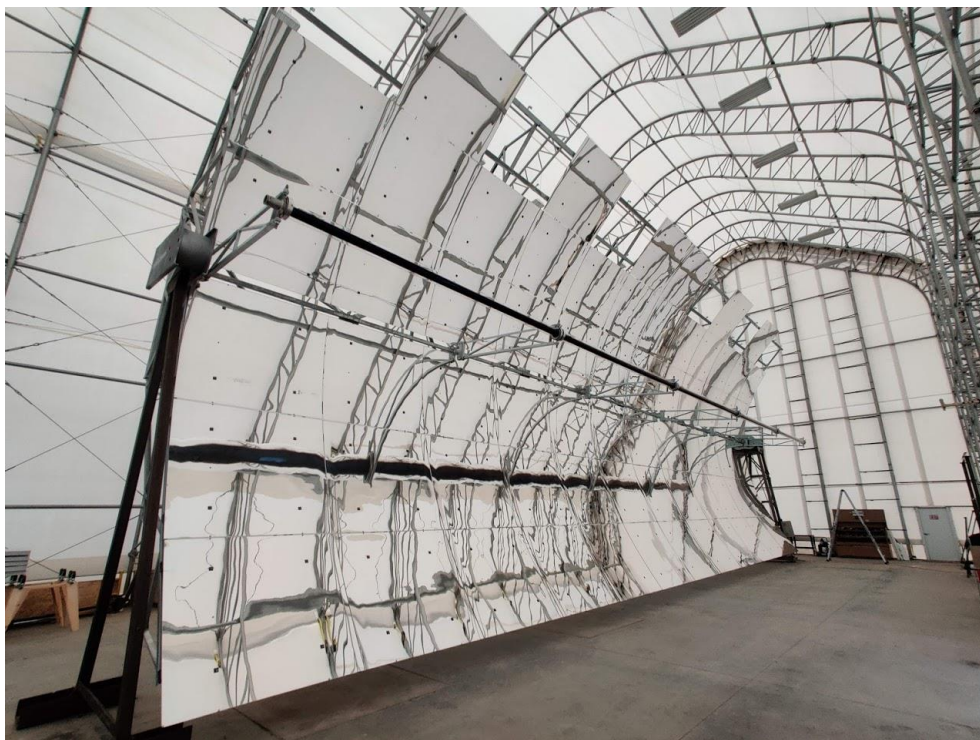
Figure 24. Picture of SunBeam™ module with HCE installed
