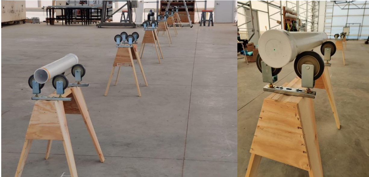
Figure 22. HCE welding stands aligned with jig and laser
