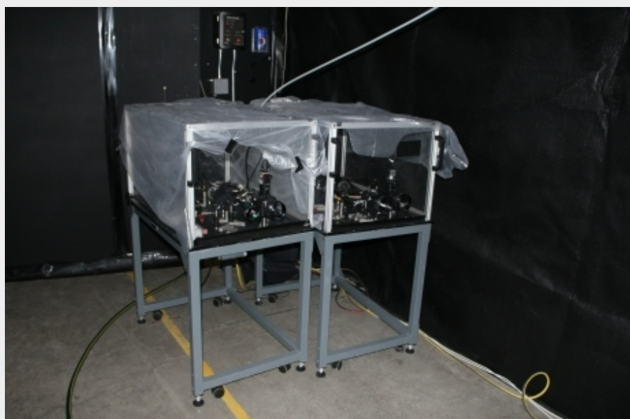
Positive pressure dry boxes are used protect instruments.
