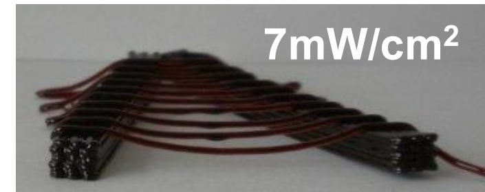
Printing of acrylate/epoxy UV/thermal dual-cure system
