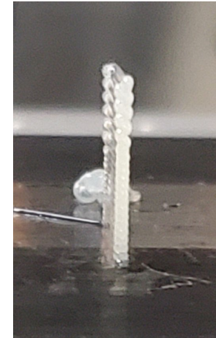
Printing of acrylate/epoxy UV/thermal dual-cure system
