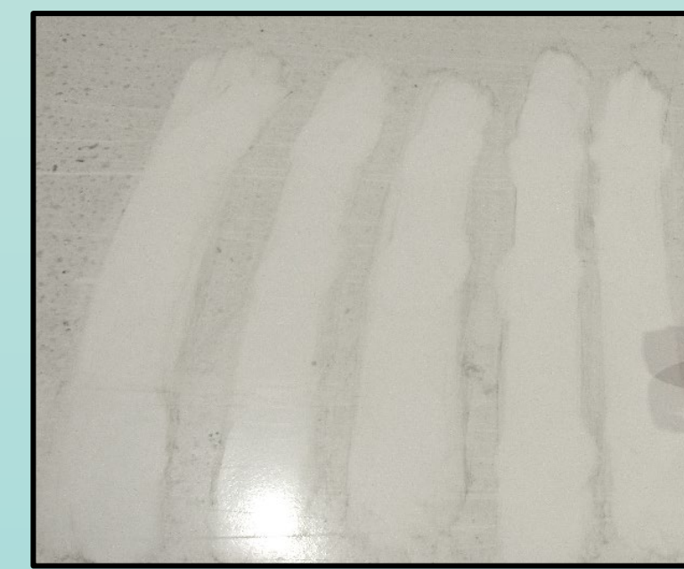
Fig. 6 – Photograph on the top of the container after spot cleaning to measure with the ET-100 and 410-Solar
