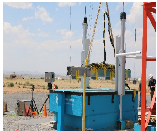
Figure 3: Surrogate assembly in basket before 30-cm drop onto unyielding target.
