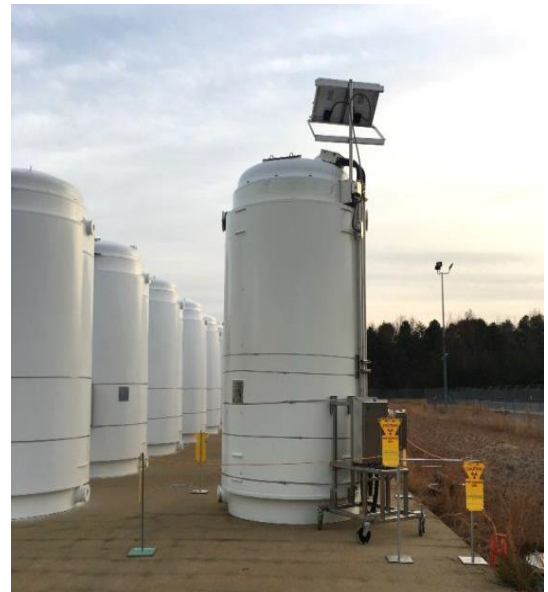
Figure 1; Loaded TN-32 for the High Burnup Demo at North Anna NPP. The solar panel is powering the 63 thermocouples inside the canister. Photo Credit: North Anna NPP
