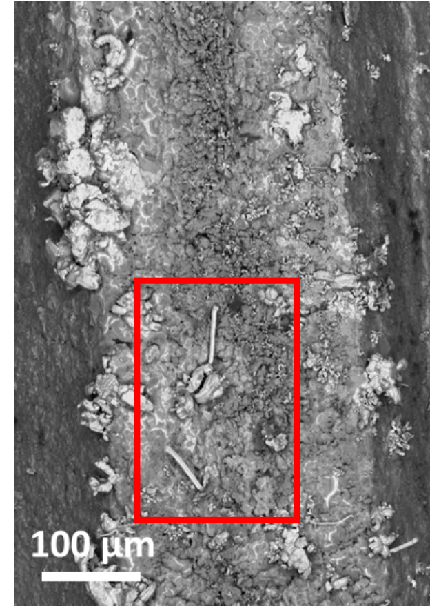
SEM BSE image on the crest of a thread (right) with a box indicating where long, straight whiskers have grown
