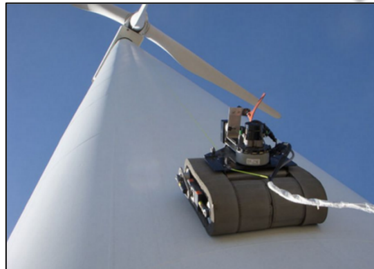
Robot with On-Board NDI System and Camera(s) for Real-Time Assessments
