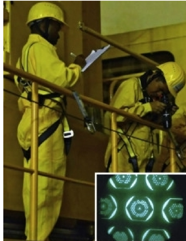
IAEA Inspectors using ICVD to detect Cerenkov glow from Spent Fuel Assemblies: Typical Cerenkov glow from VVER fuel seen in inserted photograph
