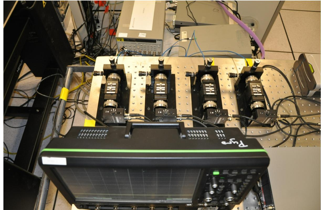
Infrared pyrometry fielded next to VISAR
