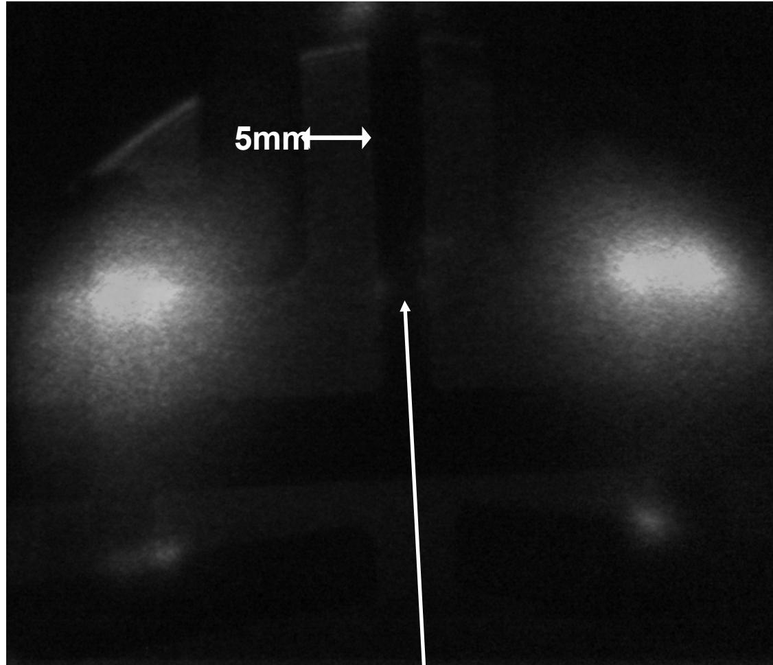
“Bright” wisps on cathode at rough height of upper anode level
