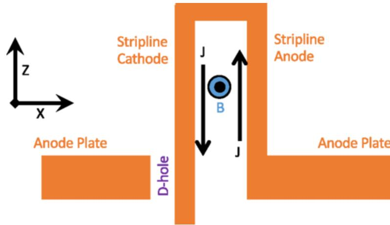
Strip-line flyer plate geometry used on the Z-machine for dynamic material property experiments
