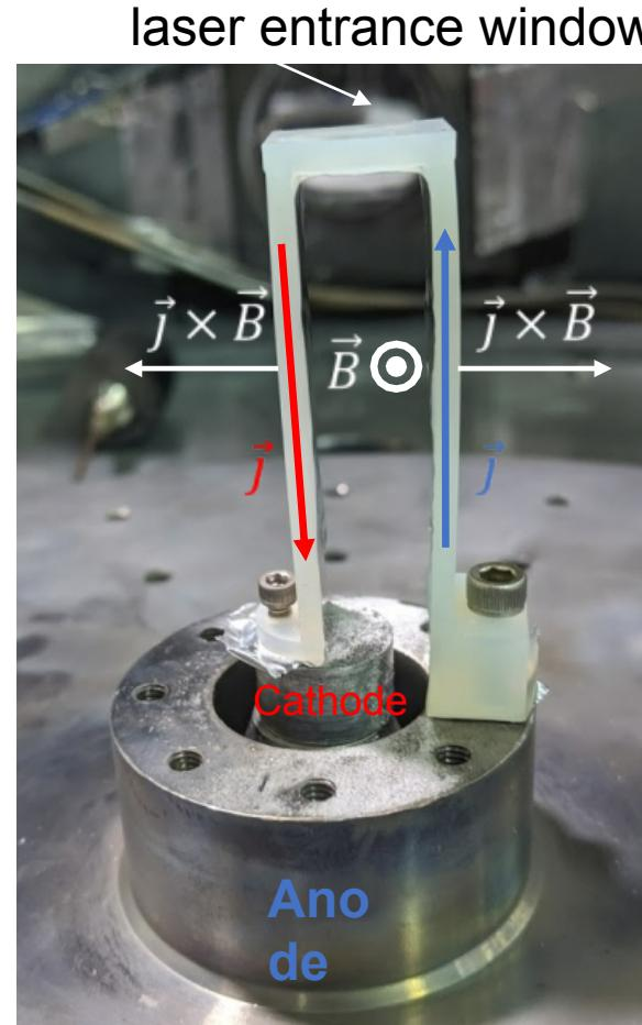
Target in situ inside MAIZE vacuum chamber
