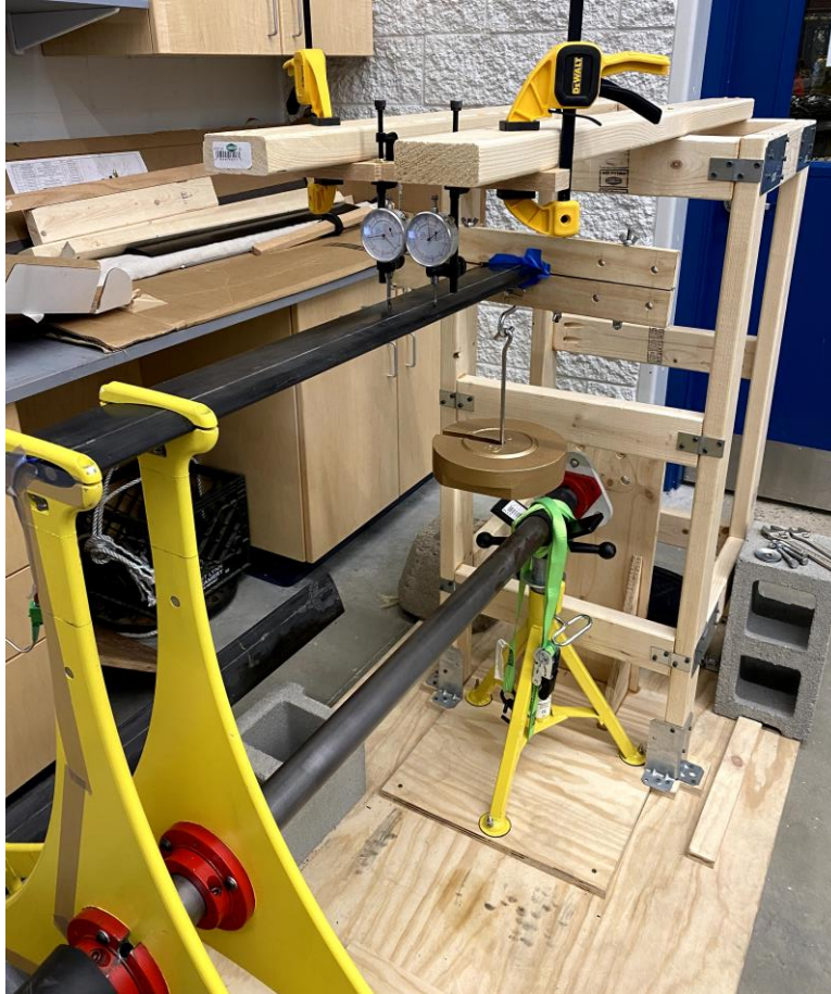
Figure 5: Calibration testing for carbon foil turbines with strut separation = 0.123m
