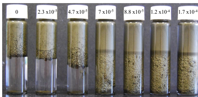
Figure 26. Effect of Span 80 in moles/l on the use of KAX-treated chalcopyrite as surfactant for emulsification.
