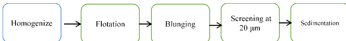
Figure 81. Flowsheet diagram of the sample preparation.
