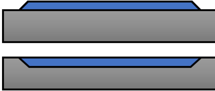
Figure 23. Coating strategies for localized coatings. Top: deposited coating without groove or blend. Bottom: grooved and blended coating.
