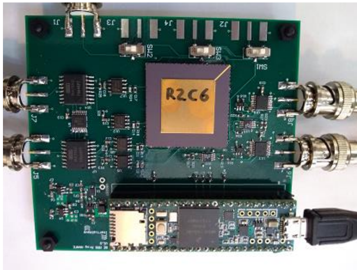
Figure 32: InertialWave Analog Frontend electronics board with attached LCC vacuum packaged GE MRG
