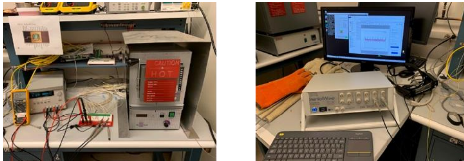
Figure 66 Test setup with 300°C chamber, probe connections to test system (outside chamber), and test equipment
