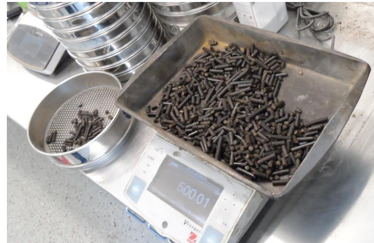
Weighing pellet sample for PDI (Pellet Durability Index) test.
