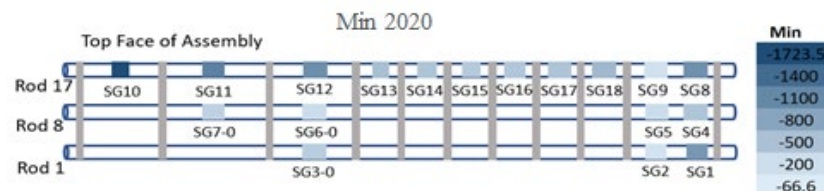
Figure 6-3. Peak Axial Strain Values (top) and Color Maps of the Peak Strain Values (bottom) in the 30 cm Drop Test of Full-Scale Surrogate Assembly.
