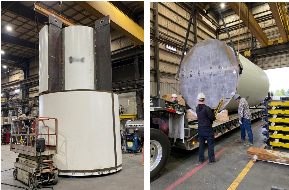
Figure 3-15. Partially Assembled Cask (left) and Fully Assembled Cask (right) Loaded on the Truck for Transport to UCSD (CA).
