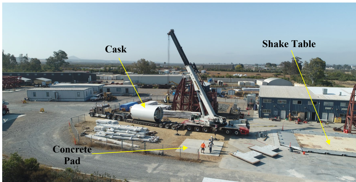
Figure 3-16. Cask Arrival to the Shake Table Facility at the UCSD.
