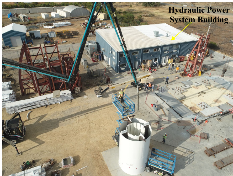
Figure 4-1. Vertical Cask Mockup at the LHPOST6 (UCSD).
