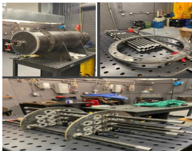
Figure 5-10. Heat exchanger undergoing pressure testing (top left), stainless steel tubes before assembly (top right), and internal frame of the heat exchanger (bottom).
