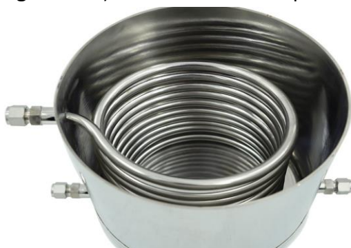
Figure 5-12. Condensing coil bucket.
