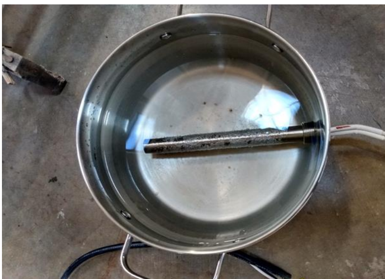
Figure 5-4. Setup for thermal desalination process demonstration using a stainless-steel pot with water heated by an electrical heating element simulating the tubes in a shell-tube heat exchanger.
