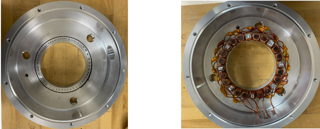
Fig. 3.C12: (Left) Stator case; (Right) Stator fixed to the stator case
