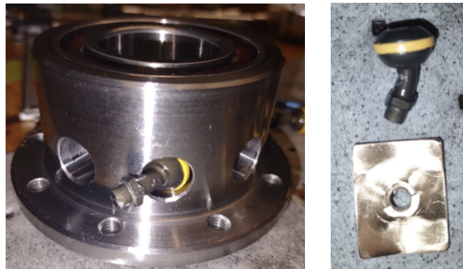
Fig. 3.C24: Collisions between piston and cylinder, and damages on the piston/slipper
