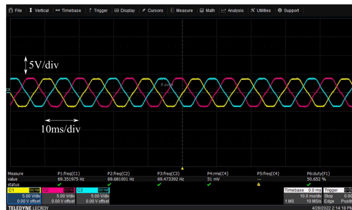
Fig. 3.C37: 3 phase voltage waveform confirms operation of the integrated machine
