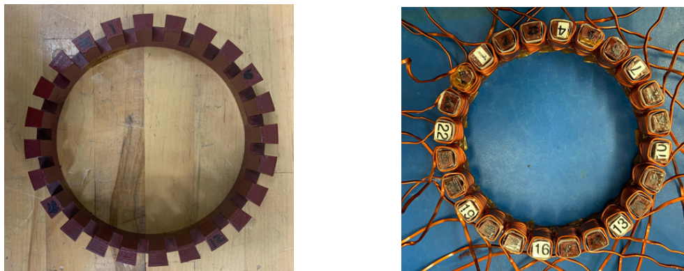
Fig. 3.C6: Electric machine stator: (left) before winding coils, (right) after winding coils.
