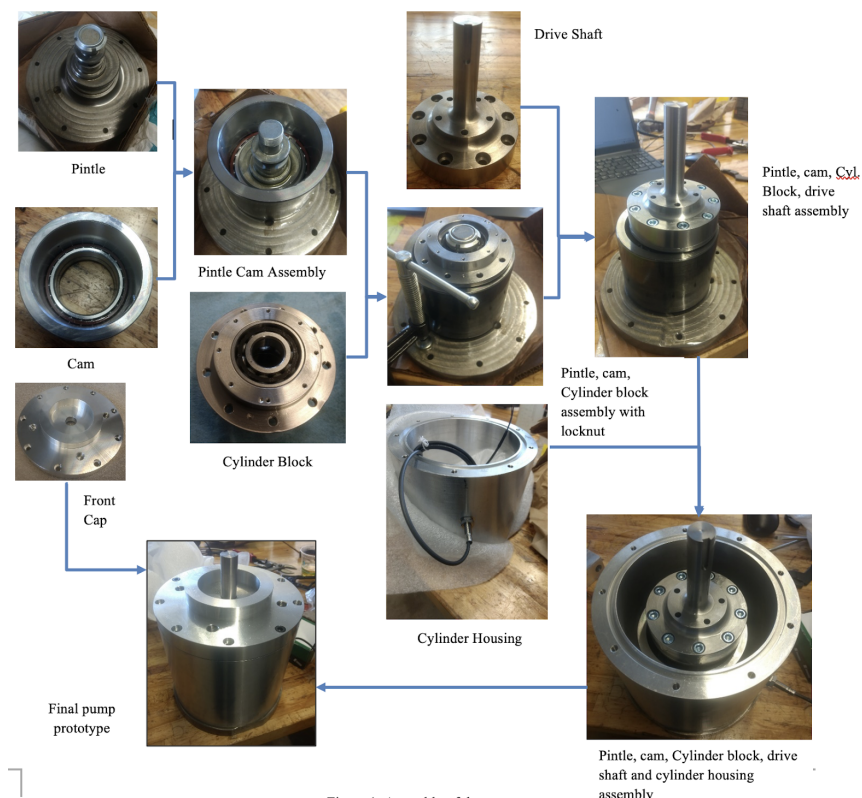
Fig. 3.C10: Hydraulic pump/motor assembly procedure
