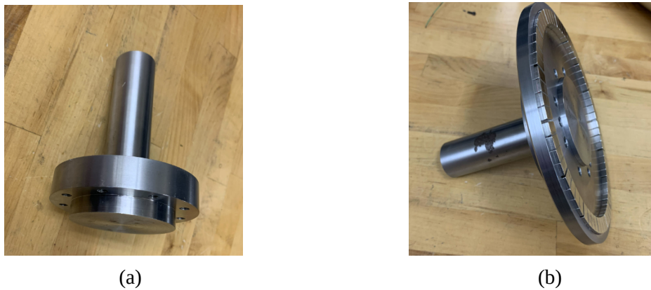
Fig. 3.C13: (a) Rotor test fixture; (b) Rotor attached to the test fixture.
