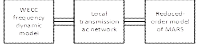
Figure 5: Test system setup in Simulink
