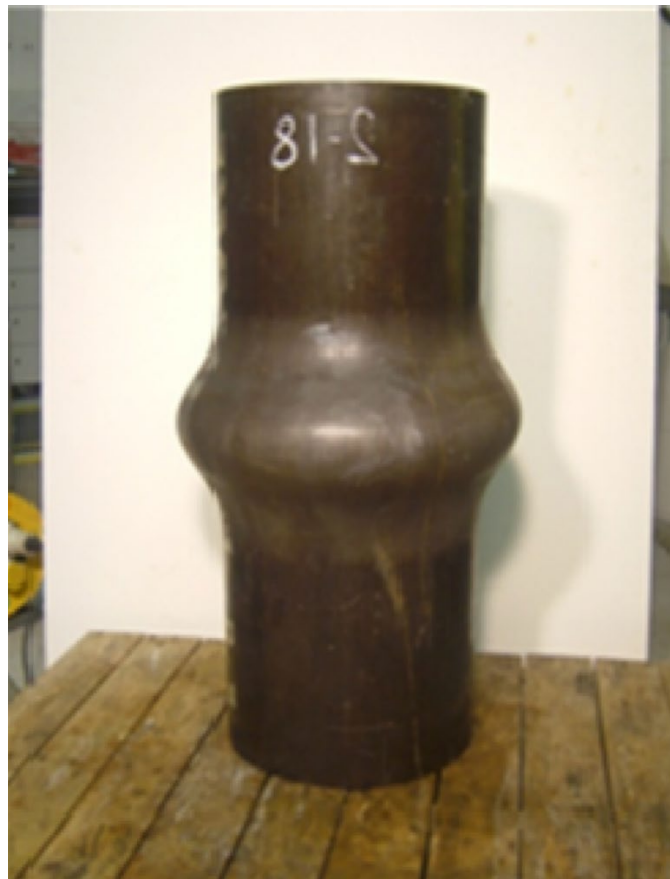
Figure 6. Representative Open-Ended Cylinder Results (Slightly below Failure Strain) From [5,9]
