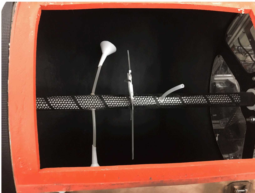
Figure 4. Inside View of Laboratory Rotating Drum. Drum contains a perforated ePTFE-lined center axle and conical reducers on sampling lines. Center of photo: mounting bracket for RH/temperature probe.
