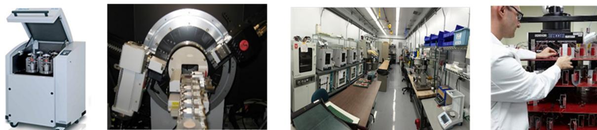
Figure 1: (from left to right) a ball mill for powder synthesis, a XRPD for powder structure analysis, a fully-equipped cell assembly facility, and a cell test station.
