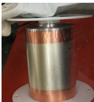
Figure 27. Photo of a roll of the 50 \mu\text{m} thick double-side lithium foil on Cu substrate for large format solid-state batteries.
