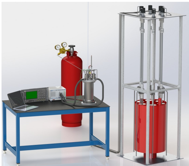
Fig. 6: Schematic of the mock-reactor; the control drums analog is located on the right, OUTSET is stationed in the middle, and the computer and controllers for the testbed are on the left.
