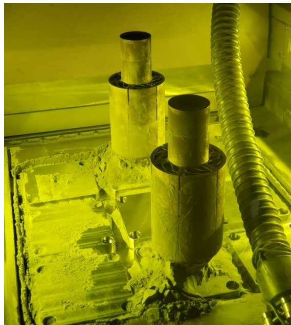
Figure 6. Parts during additive manufacturing process
