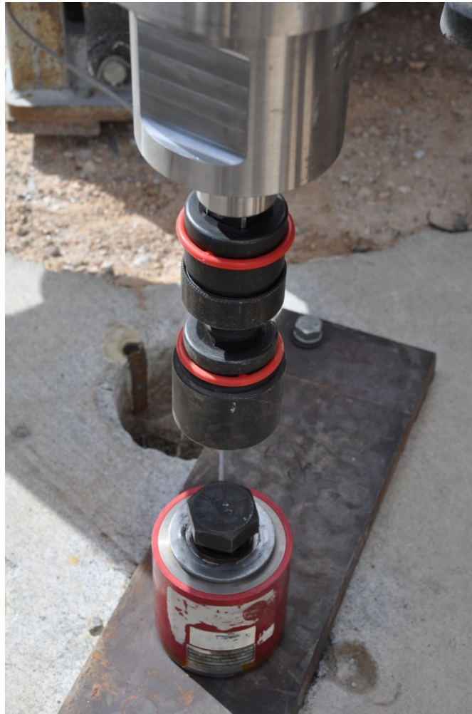
Figure 9. Load cell and bolt torque test fixture
