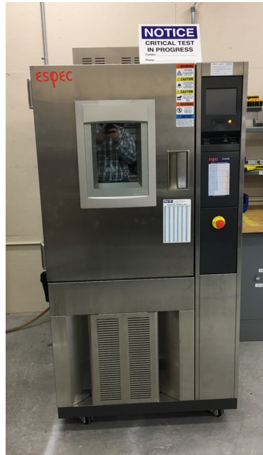
Figure 6 SNL Thermal Chamber
