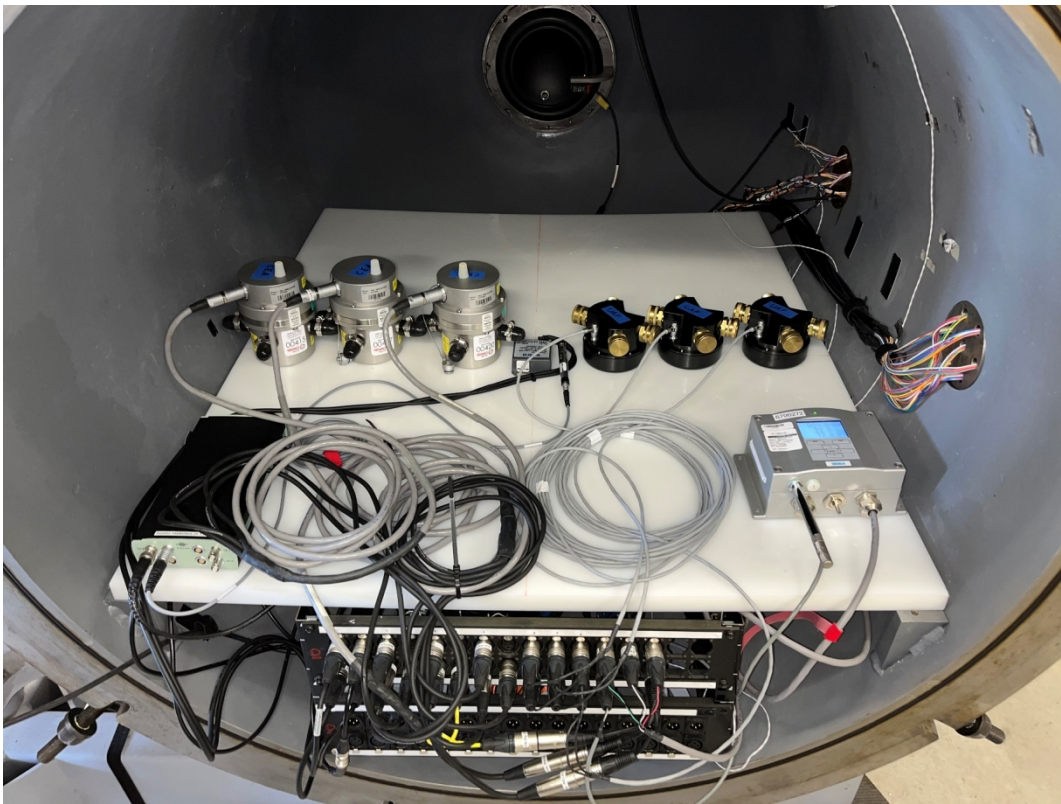
Figure 4 SNL 1400L Infrasound Chamber
