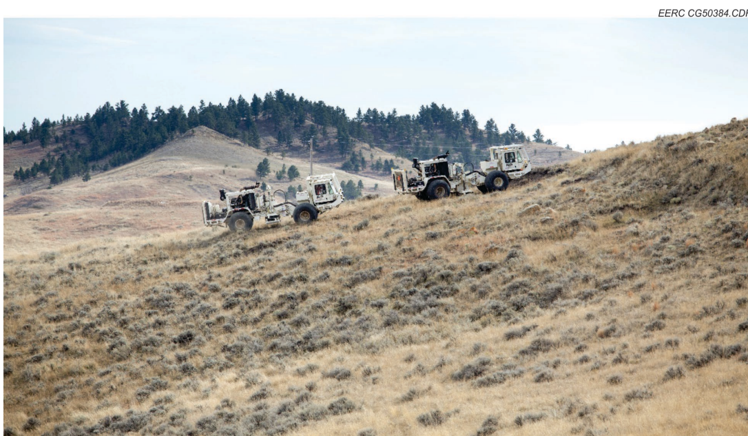
Figure 15. Vibroseis trucks are used to conduct 3-D VSP surveys in the Bell Creek Field.
