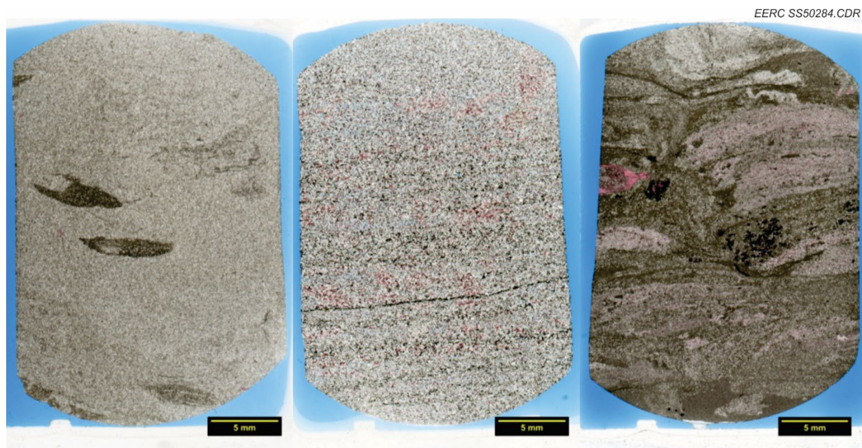
Figure 4. Whole thin-section scan demonstrating textural differences throughout the three Middle Bakken units observed in this well. Units A, B, and C are shown from left to right.
