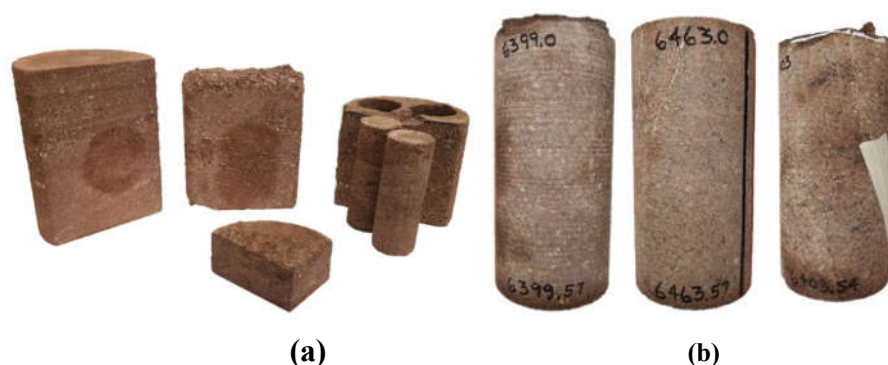
Figure 27. a) Cores of Argenta from depths between 6,296-6,299 ft. b) Cores of Precambrian rhyolite (basement rock) from depths between 6,399-6,464 ft.
