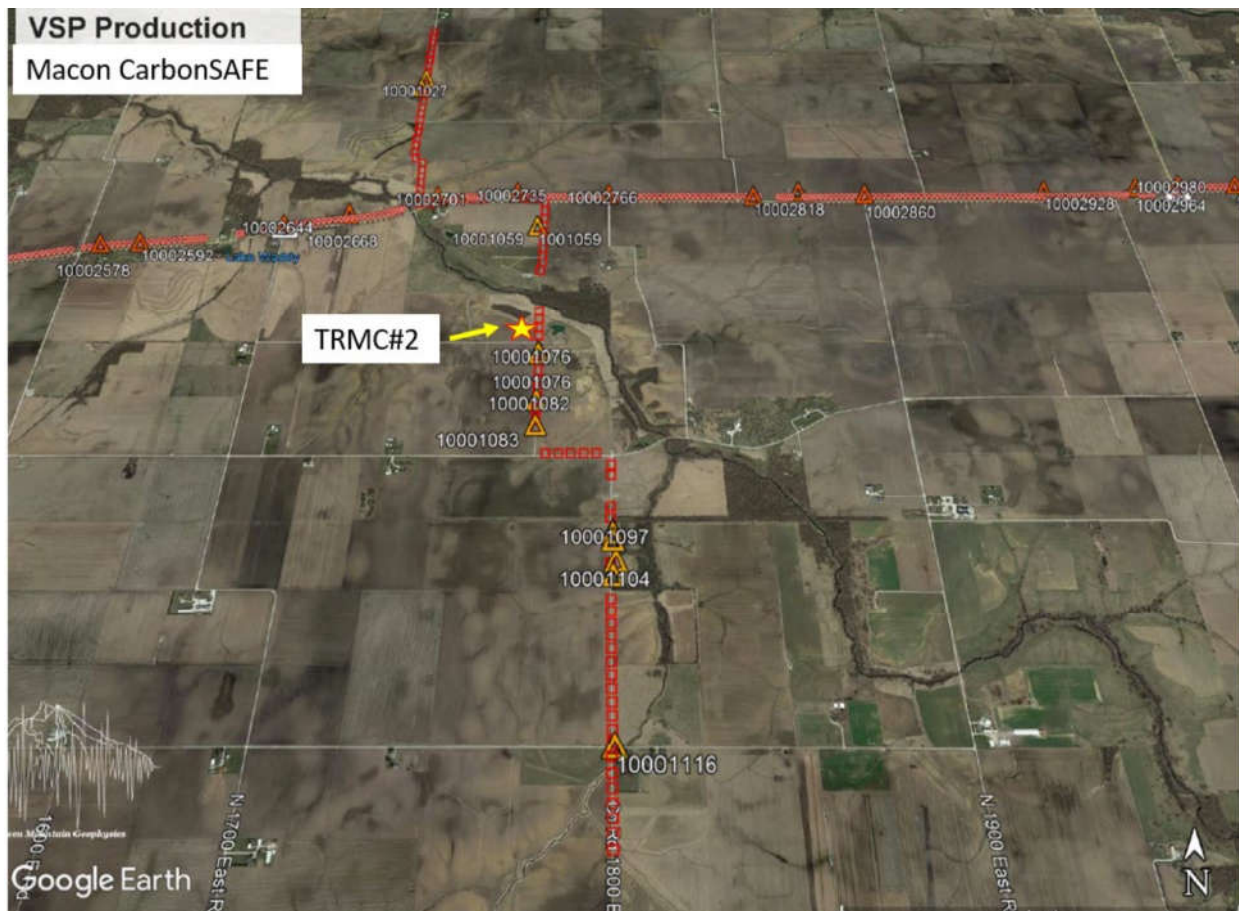
Figure 26. Location of the 2D walkaway VSP survey trending N-S and crossing the E-W 2S surface seismic survey line
