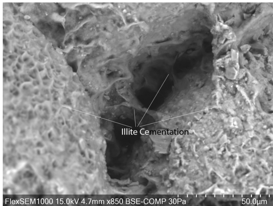
Figure 18. SEM photomicrograph of the Lower Mt. Simon Sandstone at depth of 6,285.70 ft. Clays often form pore bridges between grains.
