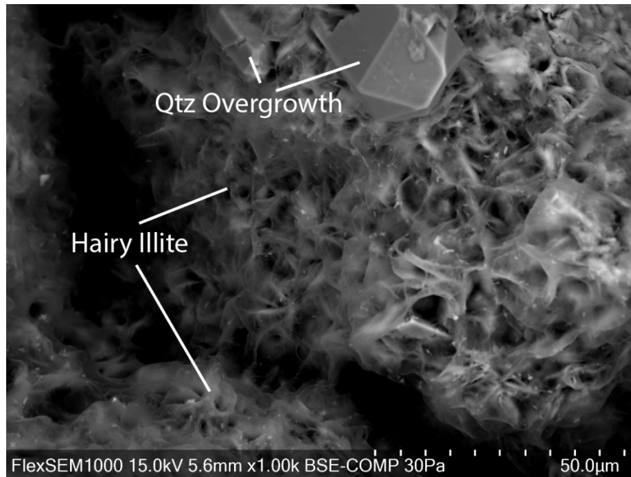
Figure 17. SEM photomicrograph of the Lower Mt. Simon Sandstone at depth of 6,249.99 ft. Abundant hairy illite lines grains, preventing pervasive authigenic quartz nucleation. Authigenic quartz is localized on small openings to the quartz grain surface between hairy illite.
