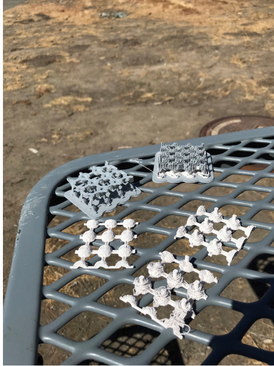
Figure 4.4 Failed attempt at 3D printing photonic crystals
