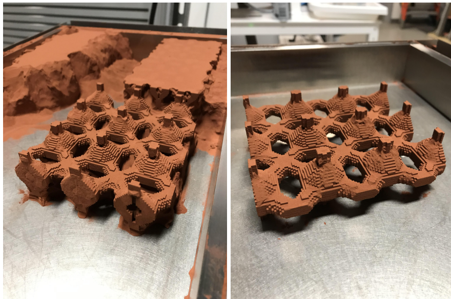
(a) Intermediate condition of part during powder removal (b) Almost final condition of part after powder removal
