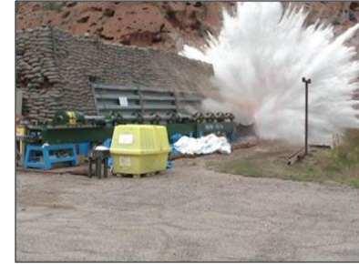
Large bore powder gun – used to measure differences in performance of weapon materials of interest
