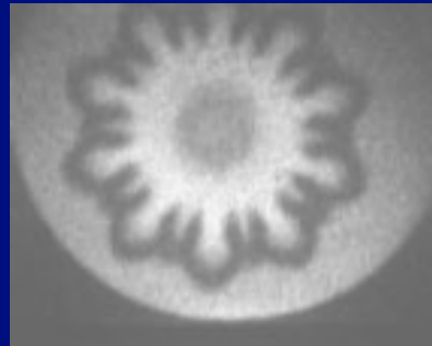
Radiograph of cylindrical Rayleigh-Taylor experiment
