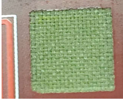
Figure 12. PCB Surface Damage at 300 W
