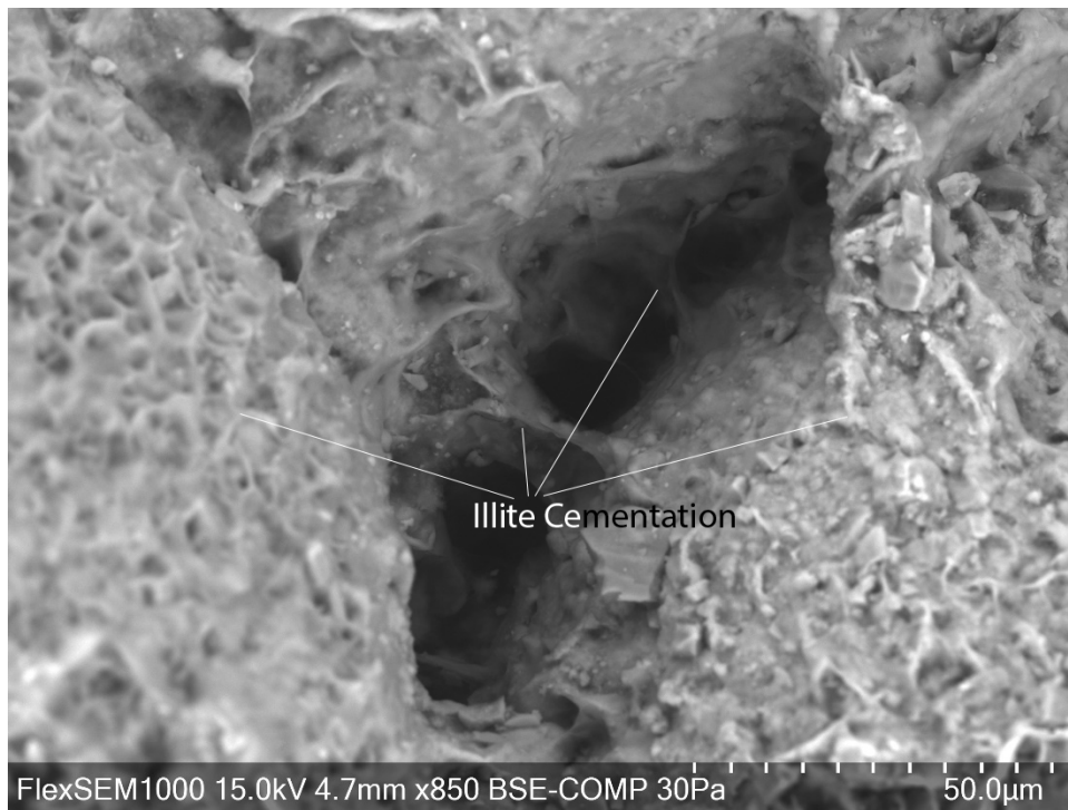
Figure 15. SEM photomicrograph of the Lower Mt. Simon Sandstone at depth of 6,285.70 ft. Clays often form pore bridges between grains.
