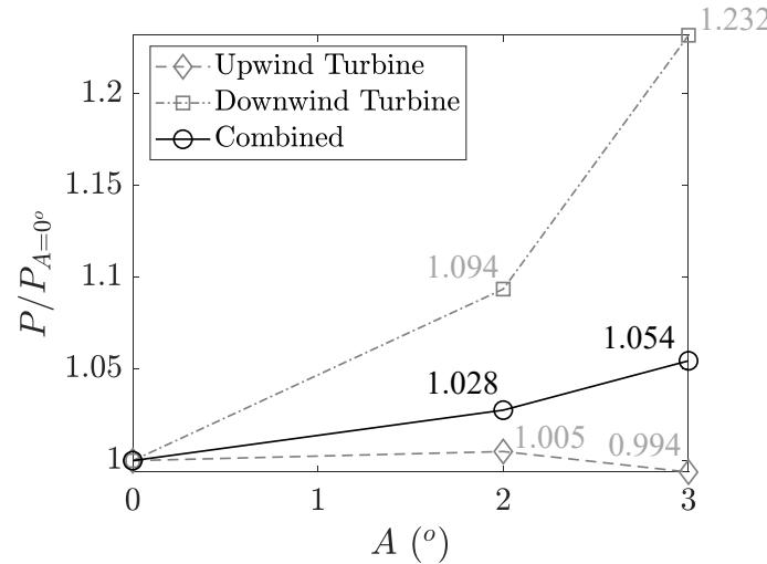
~23% increased power predicted for the second turbine at the highest pitch rate with likely increases of 10-15% power possible for a third turbine
