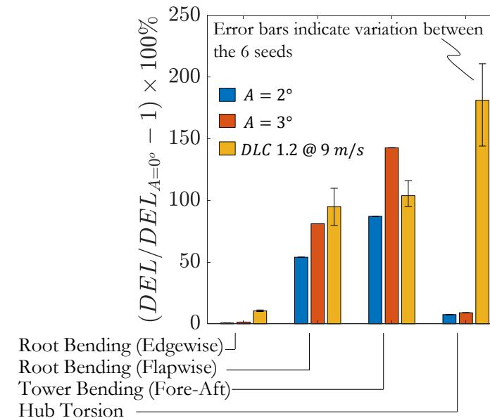
Only in one case (i.e., fore-aft tower root bending) is the damage from PBP in the stable ABL worse than the damage from the DLC 1.2 runs at a similar mean inflow velocity
