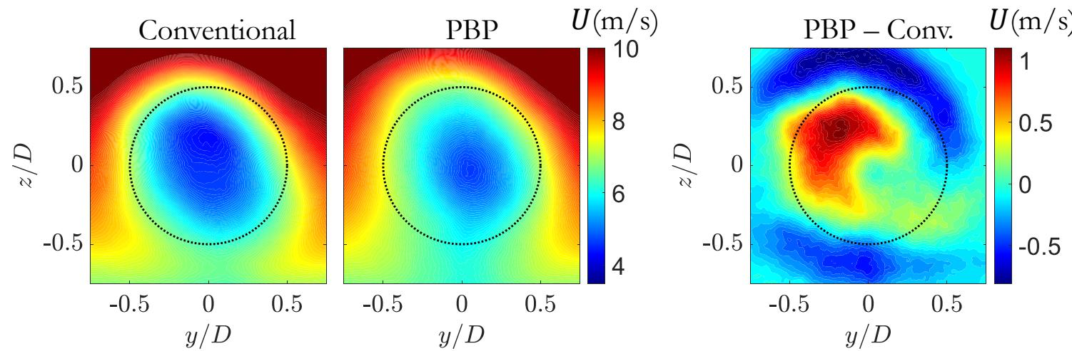
Largest velocity gain is near top of azimuth at ~75% span
