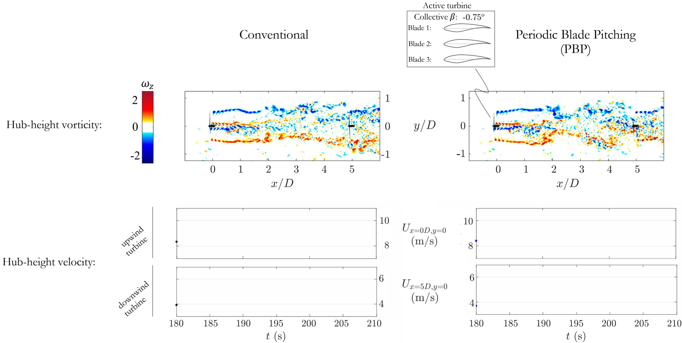
PBP amplifies coherent structures that generate mixing across the shear layers
