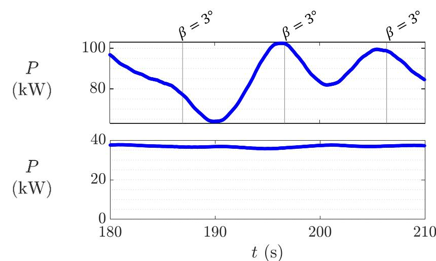
Cyclic loading from PBP  $\gg$  cyclic loading from shear/veer
