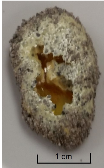
Figure 4. Small scaled 5F Test sample (dolomite) at 23.5 g was not preheated in a peri dish after cool, showing evidence of convective flow of the dark granules that were noticeable concentrated on the surface of the sample.
