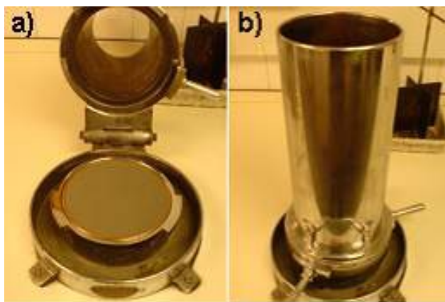
Figure 4 The hand sheet maker enables rapid evaluation of new nonwoven systems
