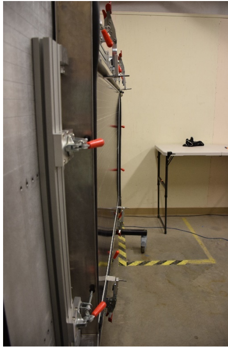
Figure 5-2: Deflection of physical module under applied pressure.
