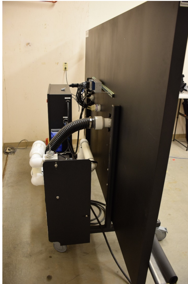
Figure 3-1: Backside of test environment showing center vacuum port.
