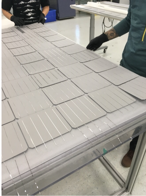
Figure 2-5: Layup of interconnected photovoltaic cells onto glass and front encapsulant.
