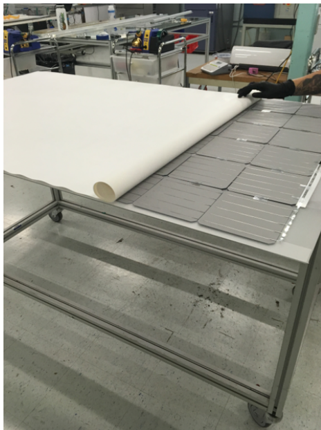
Figure 2-7: Rolling of EVA sheet over photovoltaic cells (left) and the placement of the back layer on top of the module (right).
