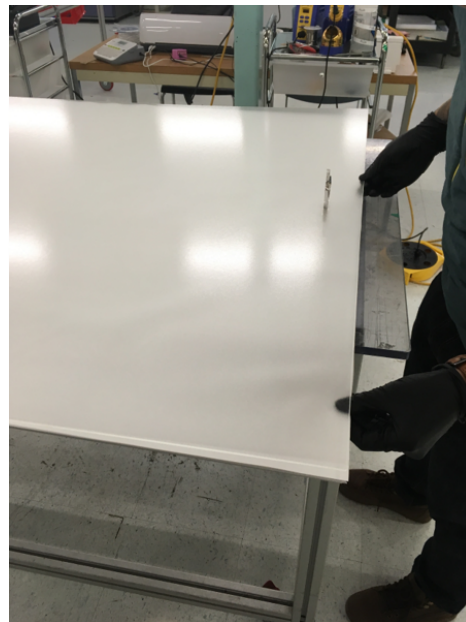
Figure 2-7: Rolling of EVA sheet over photovoltaic cells (left) and the placement of the back layer on top of the module (right).
