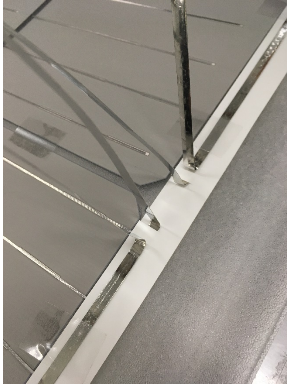
Figure 2-6: Electrical connections between photovoltaic cell rows and tabbing of connections to be fed into module junction box.
