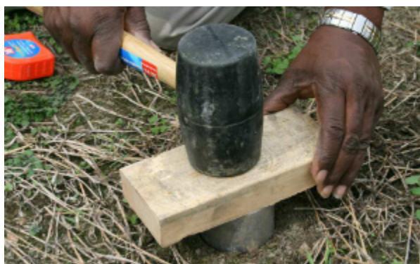
Fig 2: Bulk density measurement normally uses cored soil samples [10]
