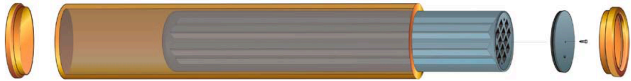
Figure 3-3. Exploded view of the canister components (from left: copper base, copper tube, insert, steel lid for insert and copper lid) (from SKB 2011, TR-11-10).
