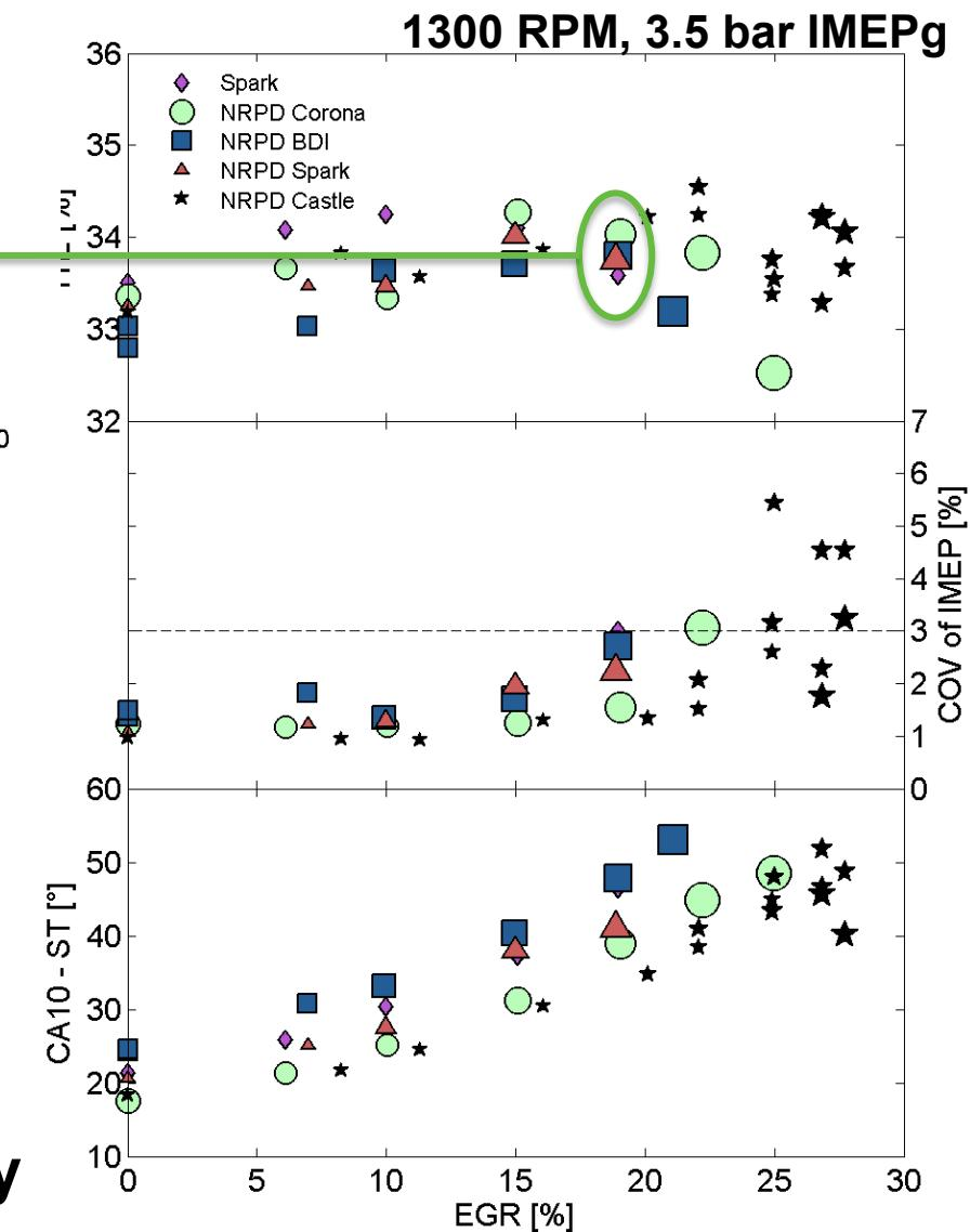
Given high discharge energies, plasma igniters likely cannot do better with current engine platform
