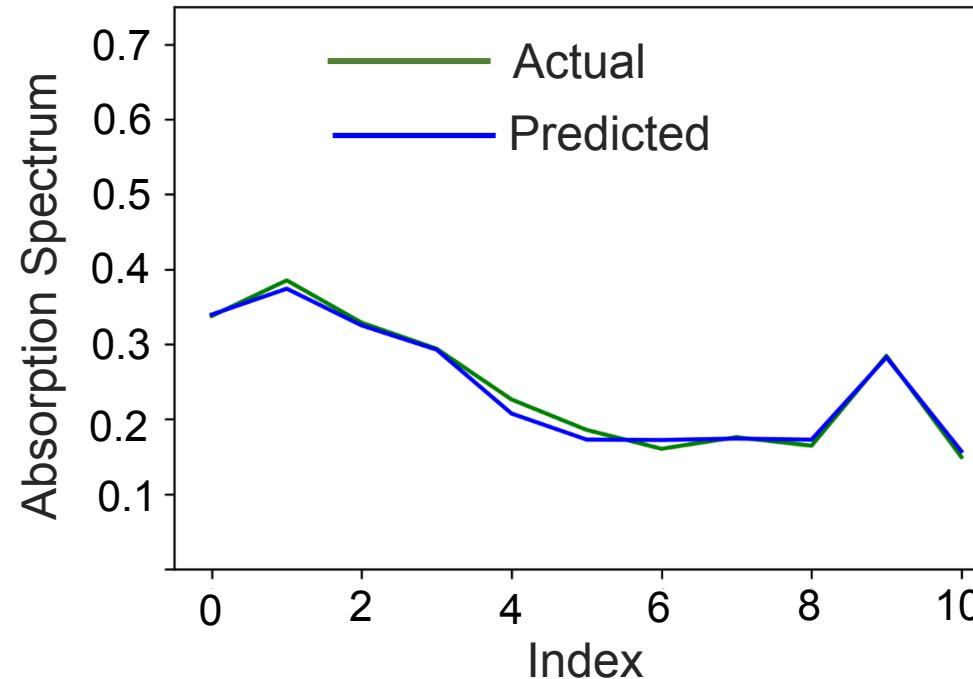
CNNs could accurately predict the absorption spectrum of metasurfaces not included in training data set.
